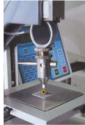
Figure 23 - Measure of a kibble's resistance to pressure
